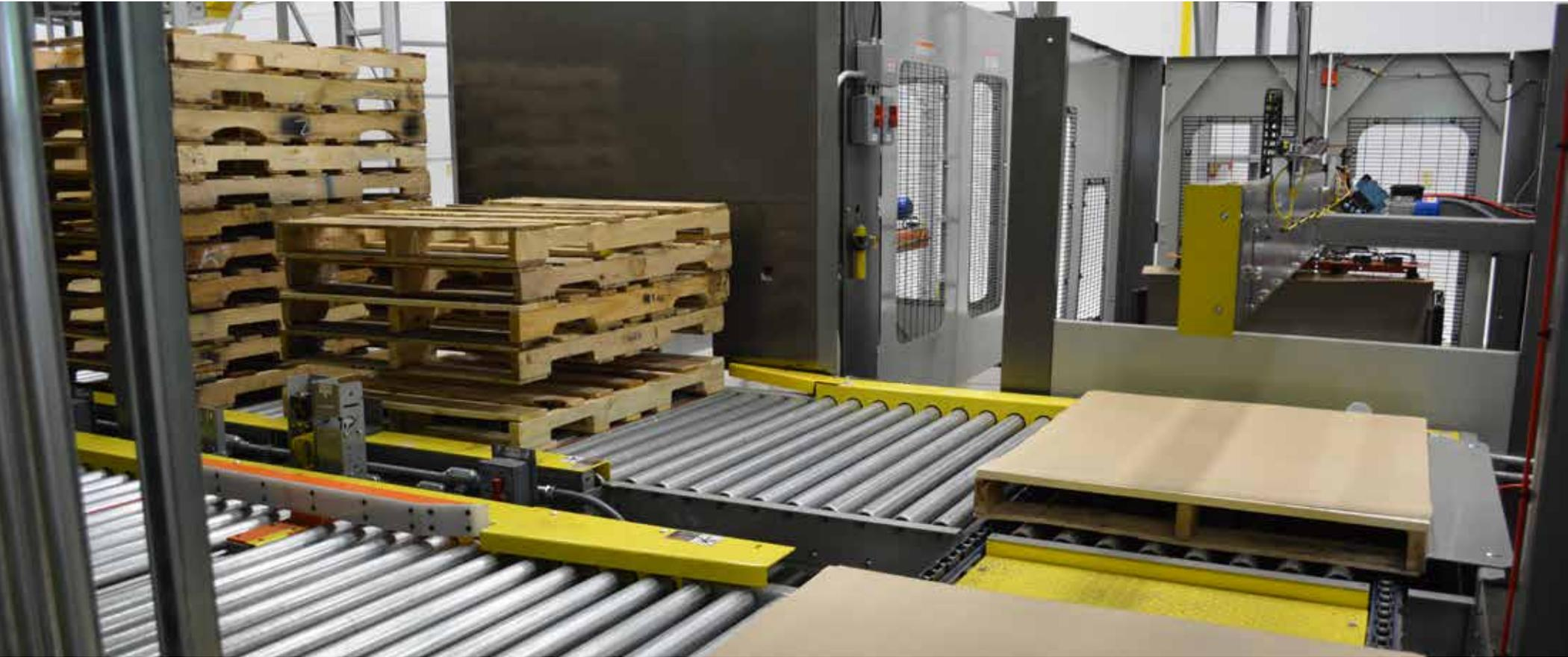
Pallets and sheets are very important parts of the palletizing process. Pallets allow for loads to be easily conveyed, moved by fork lift or stored in racks. Sheets help to stabilize the pallet load and protect the packaging during transit and storage. There are many elements impacting both pallets and sheets so it is important to select a palletizer vendor that is experienced with these factors.
