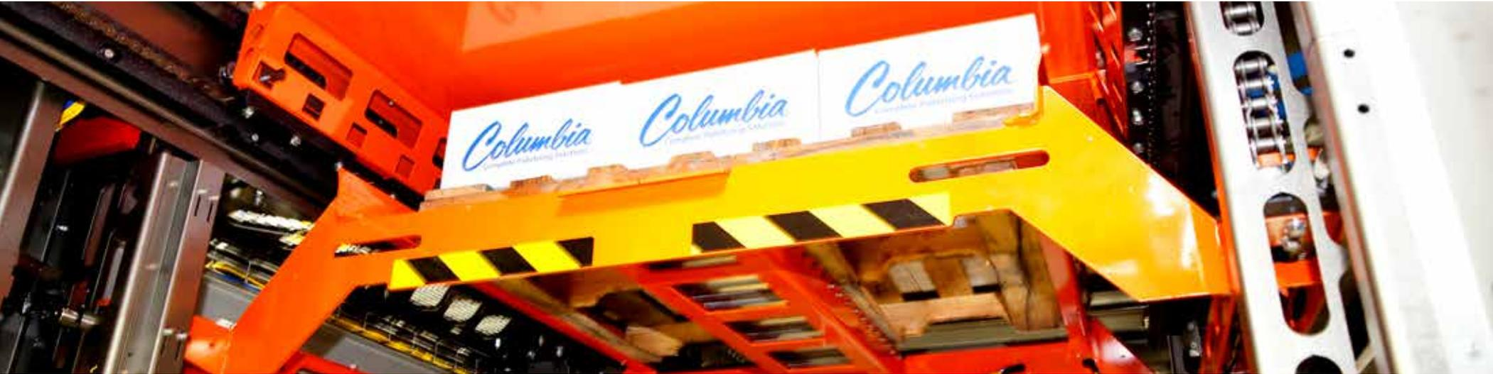
Columbia's standard safety package contains Category 3 electrical safety system including AB's SensaGuard dual circuit safety interlocks, full height light curtains and comprehensive guarding package. This safety package provides a fully guarded, Performance Level D palletizer to keep your employees safe while meeting production demands.
