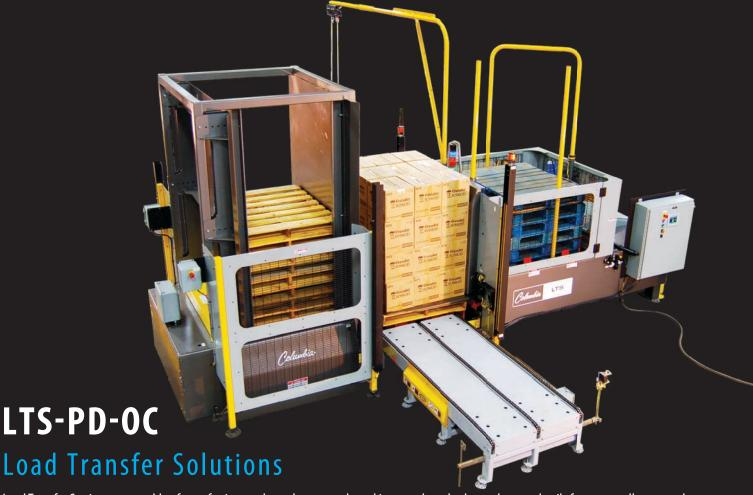
Load Transfer Stations are capable of transferring products that are packaged in cases, barrels, drums, bags and pails from one pallet to another including Plastic, Chep and GMA pallets in both receiving and shipping applications. Make your next load transfer an easy one with the LTS-PD-OC from Columbia Machine, Inc.
