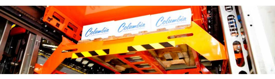
Columbia's standard safety package contains Category 3 electrical safety system including AB's SensaGuard dual circuit safety interlocks, full height light curtains and comprehensive guarding package. This safety package provides a fully guarded, Performance Level D palletizer to keep your employees safe while meeting production demands.
