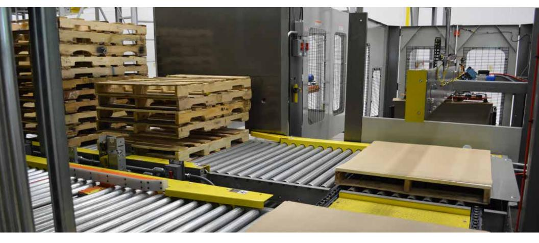
Pallets and sheets are very important parts of the palletizing process. Pallets allow for loads to be easily conveyed, moved by fork lift or stored in racks. Sheets help to stabilize the pallet load and protect the packaging during transit and storage. There are many elements impacting both pallets and sheets so it is important to select a palletizer vendor that is experienced with these factors.
